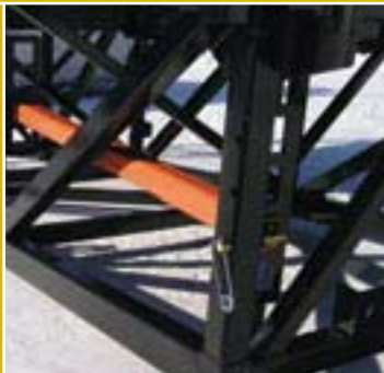
Built-in storage Modular extensions feature built-in storage for outriggers and pins.
